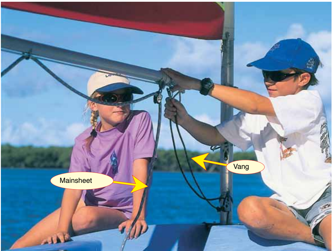
Connecting the vang — this holds the boom down when the sail fills with wind.
